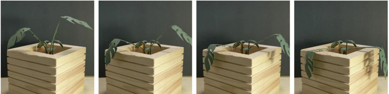
Figure 1: One of our artifacts used in the study, with the ability to move its stems up and down at a variety of speeds. Various scripted movements using this mechanism were presented to interviewees to capture their impressions on ambient-to-disruptive notifications using Shape-Changing Interfaces. Please see our supplemental video for animated examples of all movement types used in our study.
