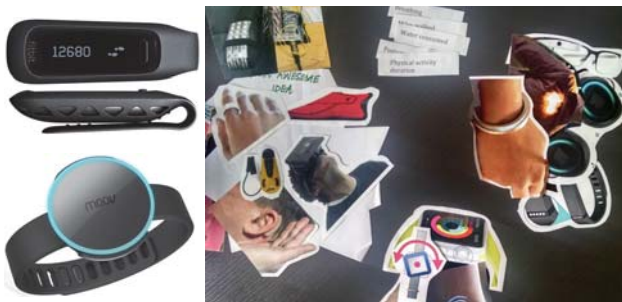
Figure 1. Left: Fitbit One (top) and Moov (bottom) devices used in the lab session. Right: Examples of prompts used for the participatory design activity: form factors (left), measurement targets (top), output (right), and input (bottom). Blank paper was also provided to sketch new ideas.
