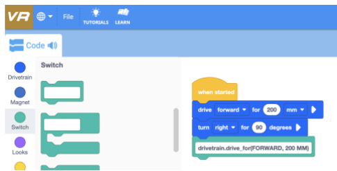
Figure 1 (left): The Switch Mode interface and the drag and drop to add Switch mode blocks to a program.
