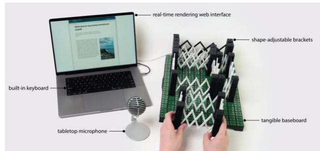
Figure 2 - System overview. TangibleSite supports accessible webpage authoring by coupling tangible layout manipulation with real-time multimodal feedback. Shape-adjustable brackets on a baseboard represent webpage elements and preserve structure across edits. Touch and audio feedback operate at both element and page levels, supporting inspection, verification, and overall layout understanding.
